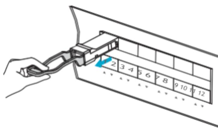
**NOTE:** If remove the module, pull the ring outward.
