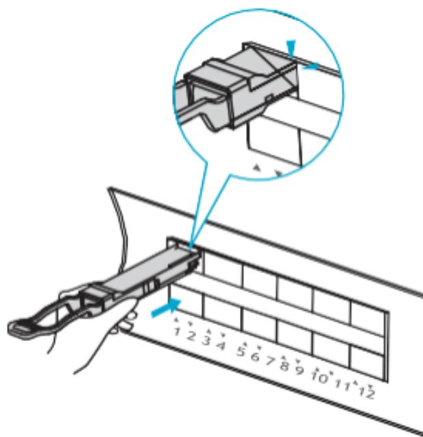
**NOTE:** When inserting into a device, please make sure the module matches the device bayonet properly. Do not push in or pull out the module with force.
