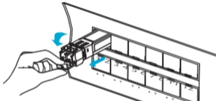
**NOTE:** If remove the module, pull the ring outward.
