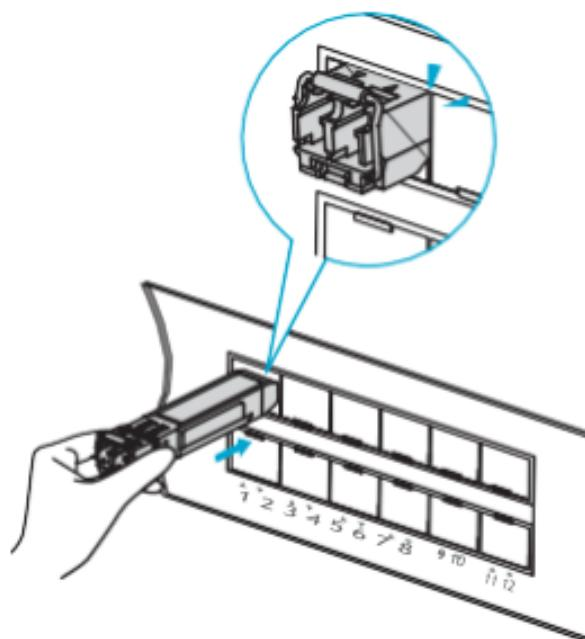
**NOTE:** Line up the module with the port and slide it gently into the port until the lock is fully seated.
